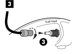
**CONNECT AND SECURE REGULATOR TO FUEL INPUT PORT** (REAR LEFT STOVE)
