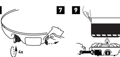
**OPEN VALVE FULLY COUNTER CLOCKWISE AND FLIP IGNITER LEVER**
