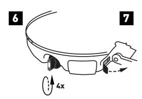
OUVRIR LA VANNE DE LA BOUTEILLE DE CARBURANT COMPLÈTEMENT DANS LE SENS ANTIHORAIRE ET FAIRE BASCULER LE LEVIER DE L'ALLUMEUR.
